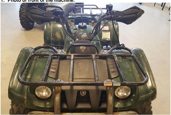
2. Remove front rack to access the power source.
