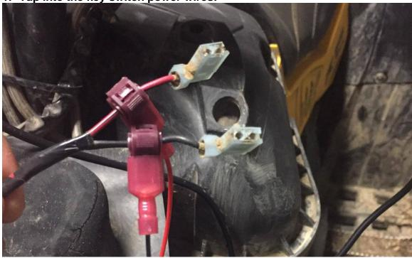
1. Tap into the key switch power wires.
