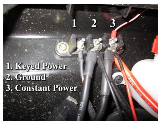
**Option Three**: Boss terminal pulse bar located on the fire wall under the front hood. This will require a bus bar wire harness (not included) and the PowerMadd terminal wire.
