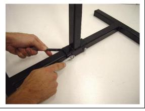
**STEP 2:** Slide the handle assembly into the center post and install the lynch pin through the hole to achieve the desired lift height.
