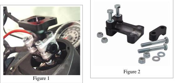
**STEP 4: Pivoting Riser Only:** Attach the handlebars to the top of the Pivoting Riser using 4 clamps, 4 long bolts and 8 washers included with kit. Make sure the handlebars are centered right to left.
