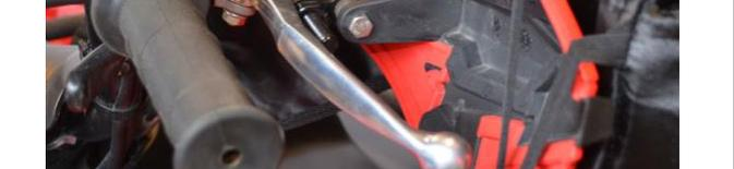
A close-up photograph showing the gauntlet fully installed on the handguard. The red elastic straps are now repositioned on the outer edge of the handguard.        |
