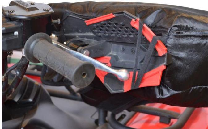
A close-up photograph showing the black gauntlet being slid onto the grey handguard. The two red elastic straps are visible, stretched over the top of the handguard. |
