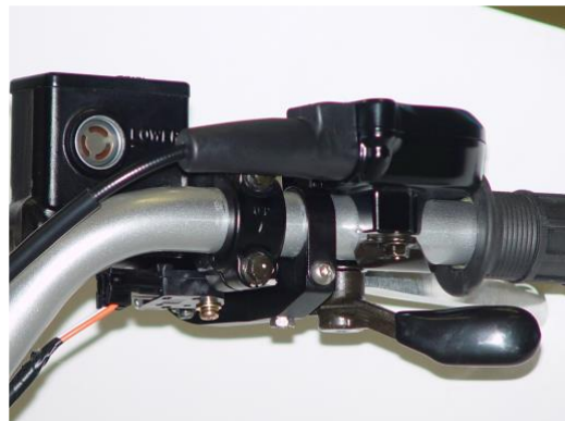
Rear view of ATV throttle - mount bracket is positioned under brake lever.
