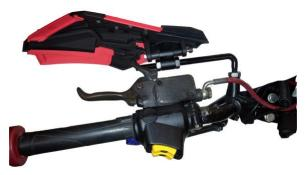
Adjustments can be made by spinning the mirror mount bracket on the bars, by turning the threaded bent rod up or down and by twisting the duck bill handguard mount. Adjust so the guard is about in the position shown in the photo and or to your personal preference. Before and after adjusting handguard check that the brake and parking brake are operational.
