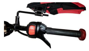
Adjustments can be made by spinning the mirror mount bracket on the bars, by turning the threaded bent rod up or down and by twisting the duck bill handguard mount. Adjust so the guard is about in the position shown in the photo and or to your personal preference.
