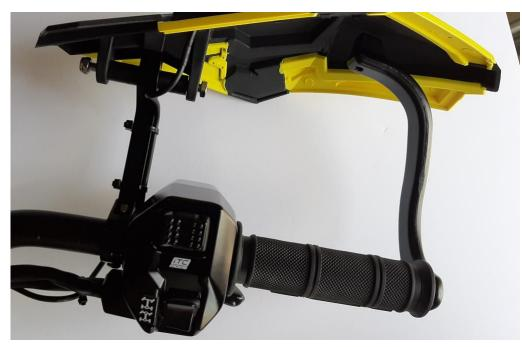
If installing the PowerMadd Hand Wrap (34253) use the instructions included with the hand wrap for information on how to install. Reference above photos for mounting location.
