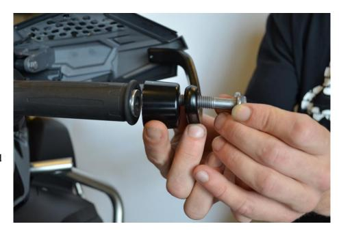
You will need to drill a ¼" hole in the Sentinel Handguard somewhere in this area of the handguard (photo 1). The exact location varies depending on how you mounted your handguards. To find the location move the Hand Wrap that you just installed on the end of your bars up to the handguard and mark this location. Use a ¼" drillbit to drill through the handguard using the marked location as a guide. **SEE PHOTO**
