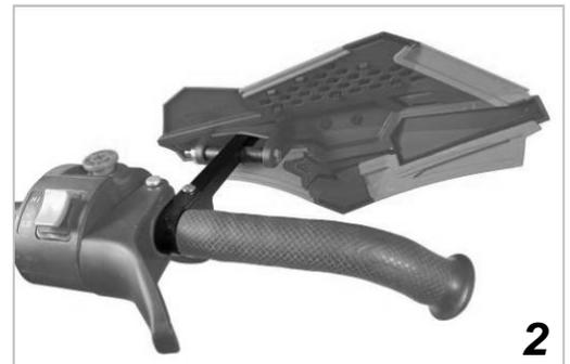
**STEP 1:** Slide the steel strap onto the handlebars. Any wires should go outside the strap.
